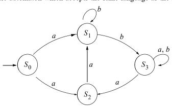
10. Find the output string corresponding to an input string aabbb for the FSM, where
